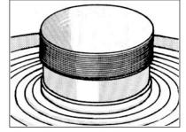
The High Temperature Voice Coil assures absolute climatic stability and great mechanical strength together with much improved power handling capacity.
