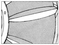
The Girdacoustic Cone improves frequency and transient response, gives much increased power handling capacity and greater mechanical stability.
