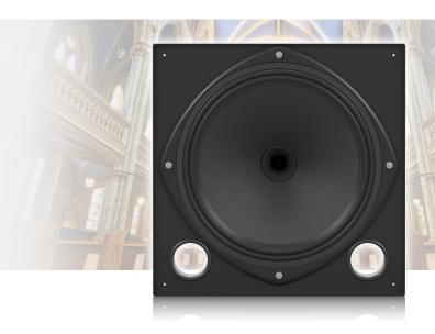
The CMS 1201DC is a full bandwidth 800-Watt high sensitivity loudspeaker that utilises our proprietary 12" Dual Concentric point-source driver, which delivers consistent broadband directivity (90° conical) with enhanced intelligibility – plus highly accurate and linear response.
