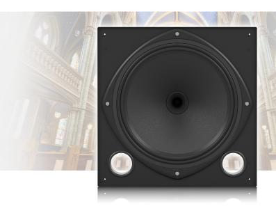
The CMS 1201DCT is a full bandwidth 800-Watt high sensitivity loudspeaker that utilises our proprietary 12" Dual Concentric point-source driver, which delivers consistent broadband directivity (90° conical) with enhanced intelligibility – plus highly accurate and linear response.
