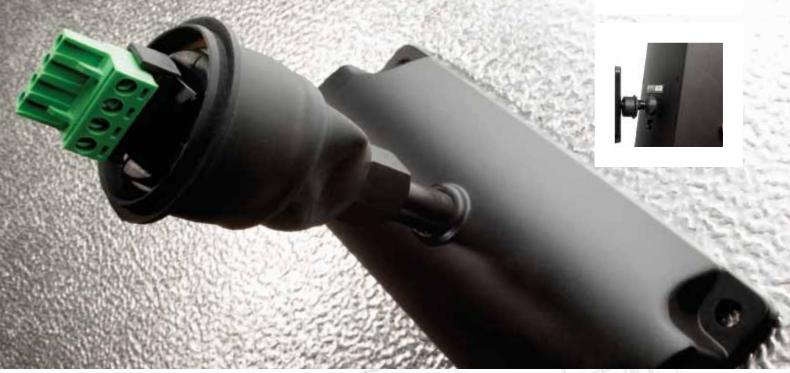
A recess on the rear of the enclosure contains the Euroblock connector socket which completes the signal path when the speaker is offered up to the bracket and pushed into place. The speaker may then be swivelled into the desired angle for optimum coverage before tightening the locking collar. A secondary support line can be secured to the tie back point and the rubber weather-sealing boot located.
