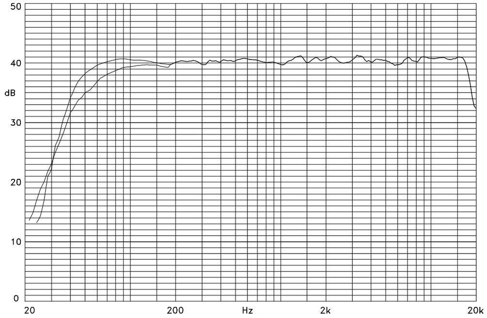
Figure 3. System 800A. Anechoic response. LF contour ON & OFF
