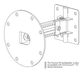
The V6 can be wall or ceiling mounted by using the V8B bracket which is designed to offer the maximum flexibility in selecting desired angles.
