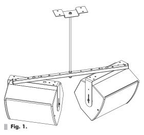
The VCS ceiling saddle available in both black and white finishes, and is to be used in conjunction with the V6Y, VCB2, VCB4 and a length of M10 threaded rod (not supplied by Tannoy Limited). The VCS ceiling saddle allows the Tannoy V6 loudspeaker to be suspended at a user defined distance from the ceiling as shown in Figure 1.
