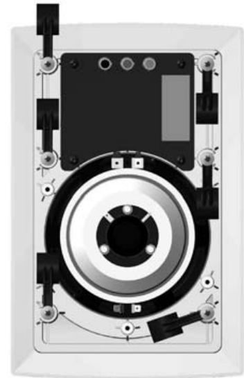
Fig 12: clamps in preinstall position
